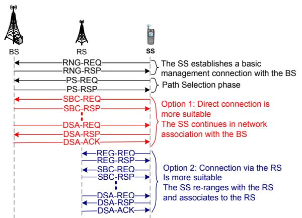
Fig. 3. Proposed message exchange during the association process when BS signal is the better
