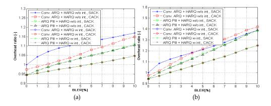
Fig. 11. ARQ & HARQ Overhead vs. BLER for ARQ\_Block\_Size = 16 B, PDU Size = 1, Size of user data = 1024 B/frame, 4 HARQ retrans., HARQ Type: IR, 1 hop (a) / 3 hops (b)
