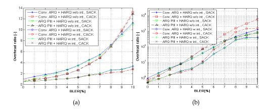
Fig. 13. ARQ & HARQ Overhead vs. BLER for ARQ\_Block\_Size = 16 B, PDU Size = 16, Size of user data = 1024 B/frame, 4 HARQ retrans., HARQ Type: IR, 1 hop (a) / 3 hops (b)
