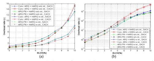
Fig. 7. ARQ & HARQ Overhead vs. BLER for ARQ\_Block\_Size = 16 B, PDU Size = 16, Size of user data = 1024 B/frame, 4 HARQ retrans., HARQ Type: CC, 1 hop (a) / 3 hops (b)
