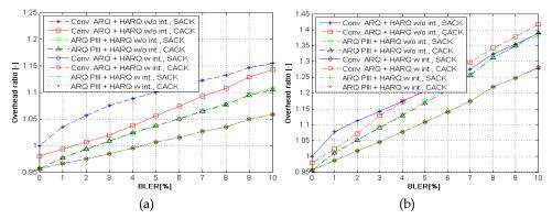
Fig. 5. ARQ & HARQ Overhead vs.BLER for ARQ\_Block\_Size = 16 B, PDU Size = 1, Size of user data = 1024 B/frame, 4 HARQ retrans., HARQ Type: CC, 1 hop (a) / 3 hops (b)
