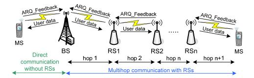
Fig. 4. Link level simulation scenario
