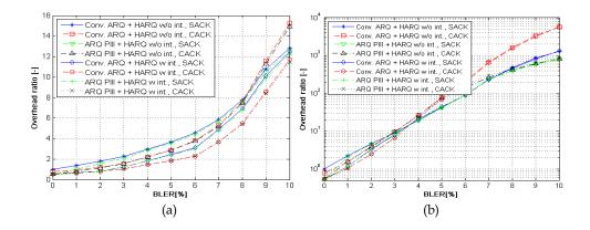
Fig. 10. ARQ & HARQ Overhead vs. BLER for ARQ\_Block\_Size = 16 B, PDU Size = 16, Size of user data = 1024 B/frame, 2 HARQ retrans., HARQ Type: CC, 1 hop (a) / 3 hops (b)
