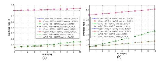
Fig. 12. ARQ & HARQ Overhead vs. BLER for ARQ\_Block\_Size = 1024 B, PDU Size = 1, Size of user data = 1024 B/frame, 4 HARQ retrans., HARQ Type: IR, 1 hop (a) / 3 hops (b)
