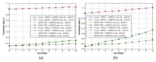
Fig. 15. ARQ & HARQ Overhead vs. BLER for ARQ\_Block\_Size = 1024 B, PDU Size = 1, Size of user data = 1024 B/frame, 2 HARQ retrans., HARQ Type: IR, 1 hop (a) / 3 hops (b)
