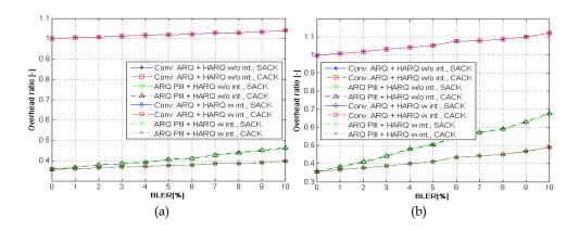
Fig. 9. ARQ & HARQ Overhead vs. BLER for ARQ\_Block\_Size = 1024 B, PDU Size = 1, Size of user data = 1024 B/frame, 2 HARQ retrans., HARQ Type: CC, 1 hop (a) / 3 hops (b)
